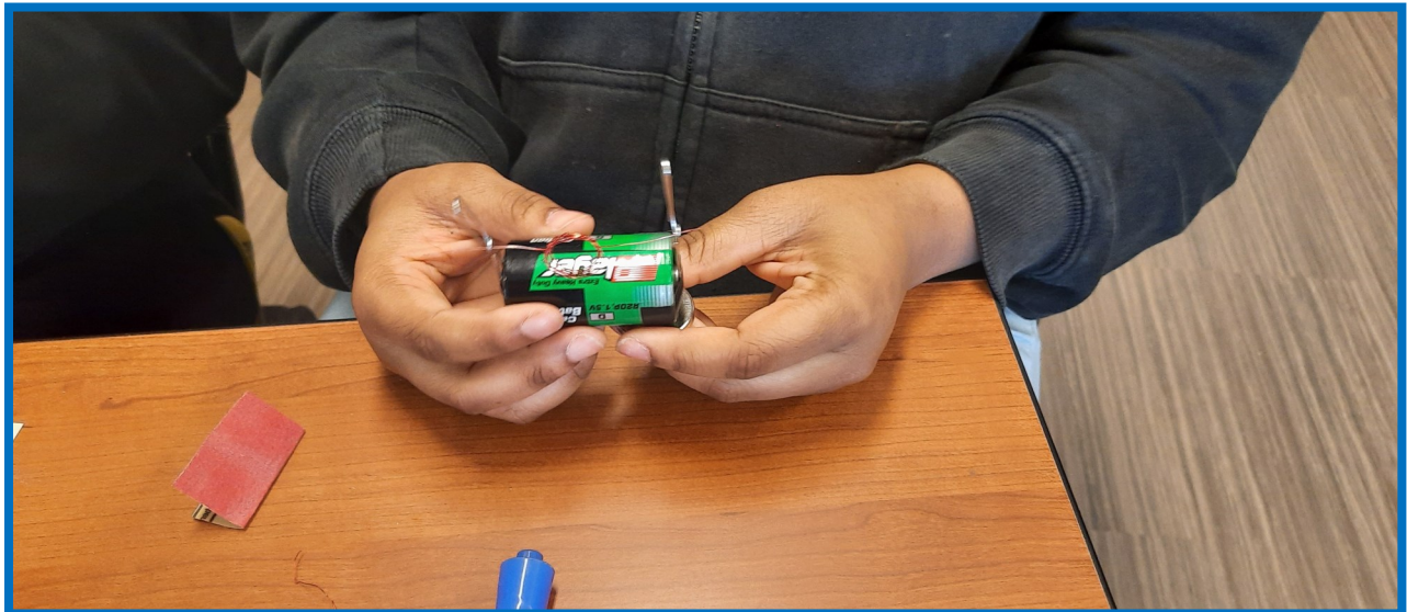
A student makes a magnetic motor. The coil makes electrical contact with the paperclip, allowing a current to run through the coil. The coil is an electromagnet.
